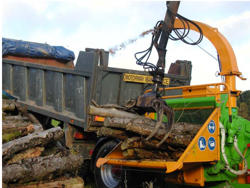
Figure 2 Chipping wood with a Heizohack HM8400
